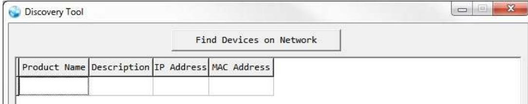
3. By clicking on one of the listed devices you will be presented with the network details of that particular device. If you choose, you can alter the static IP network settings for the device or switch the unit into DHCP mode to automatically obtain proper network settings from a local DHCP server. To switch to DHCP mode, please select DHCP from the IP mode drop-down, then click **“Save”** followed by **“Reboot”**.
